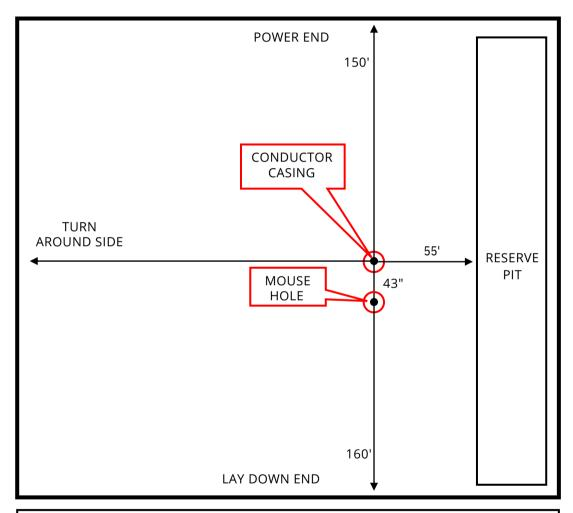
Note: Allmeasurements are from the center of the conductor casing. The mouse hole is 43" from the center of the conductor casing w/ 0° slope (angle). This rig has a top drive so the mouse hole should be a minimum of 75' deep (from ground level) with casing or liner with a minimum ID of 10". The reserve pit is a minimum of 55' from the center of conductor casing.
