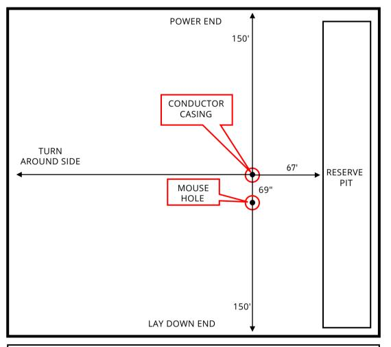
Note: <u>All</u> measurements are from the center of the conductor casing. The mouse hole is 69" from the center of the conductor casing w/  $0^{\circ}$  slope (angle). This rig has a top drive so the mouse hole should be a minimum of 75' deep (from ground level) with casing or liner with a minimum ID of 10". The reserve pit is a minimum of 67' from the center of conductor casing.
