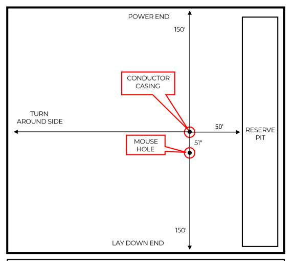
Note: <u>All</u>measurements are from the center of the conductor casing. The mouse hole is  $51^{"}$  from the center of the conductor casing w/ 0° slope (angle). This rig has a top drive so the mouse hole should be a minimum of 75' deep (from ground level) with casing or liner with a minimum ID of 10". The reserve pit is a minimum of 50' from the center of conductor casing.
